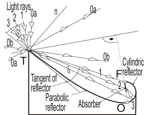
Figure 4 Light ray path toward the concentrator (the cross cut of parabolic-cylindric concentrator with one parabolic and cylindric reflector).
